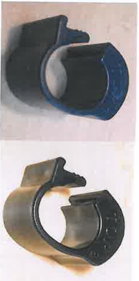
Photo 1: The tested blue and black versions of the Topigeon chipping with Hitag-S transponder
