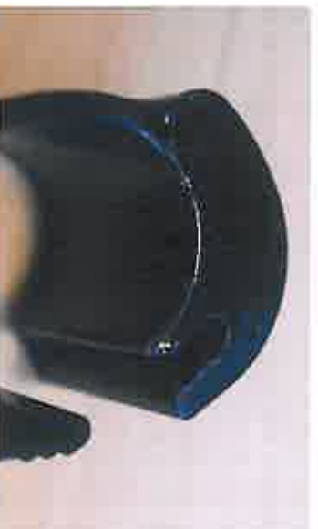
Photo 2: The transponder is placed inside the chipping and sealed with black resin
